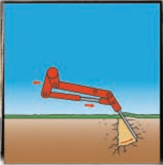
Verti-Drains adjustable parallelogram design shatters the soil, and also allows for clean Coring, on all models.
