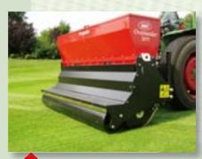
Overseeder 1275 equipped with the optional bogy wheel kit.
