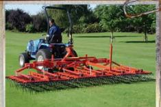
The Verti-Rake decompacts turf surfaces using thin spring-loaded flexible tines. The tines are integrated in a special protection device that will prevent the loss of tines during operation.
