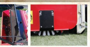
The walk-behind Verti-Top is self-driven and powered by a 6 1/2 HP engine. It is ideal to clean smaller areas.
