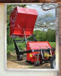
The Redexim North America Turf Tidy is one of our most versatile machines incorporating de-thatching, verticutting, flail cutting and sweeping. Turf Tidy's fully floating cutting head follows the grounds' contours, ensuring accurate cutting and pick-up. The unique turbo fan makes a clean sweep of leaves, pine needles, paper and grass clippings. The large hopper means less time emptying and its high lift allows greater clearance when tipping.
