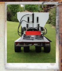
The Rink DS 1200 is a topdresser with dual spinners with a spread pattern variable up to 30 ft (10 m). The operation of the belt and spinners can be done from the tractor seat, by switching the hydraulic lever. No unnecessary drop of material takes place between stopping and operation, since the material release gate automatically closes when the belt is stopped. The spinner disks have been designed in a way that they will handle wet material very well.
