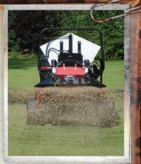
The Rink DS 800 is a topdresser with dual spinners with a spread pattern variable up to 10 m. The operation of the belt and spinners can be done from the tractor seat, by switching the hydraulic lever. No unnecessary drop of material takes place between stopping and operation, since the material release gate automatically closes when the belt is stopped. The spinner disks have been designed in a way that they will handle wet material very well.
