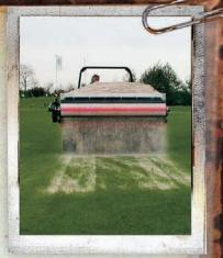
The 12 series top dressers offer you the widest brush applicator top dresser available with a smooth even spread, over 6 ft. wide. This makes the 1210 body mount spreader ideal for fitting onto your utility vehicle, as its spreading width will be outside the vehicle's wheel width. The 1210 is a trailed unit for use behind any prime mover.
