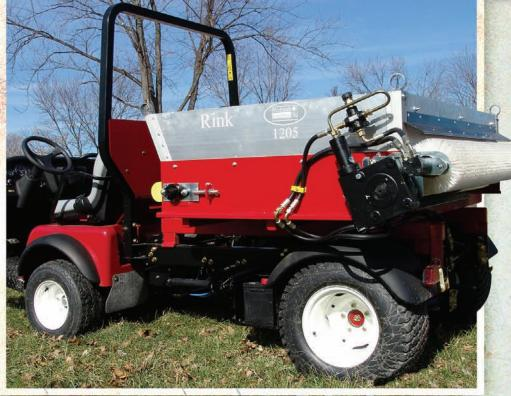
The 12 series top dressers offer you the widest brush applicator top dresser available with a smooth even spread, over 6 ft. wide. This makes the 1205 body mount spreader ideal for fitting onto your utility vehicle, as its spreading width will be outside the vehicle's wheel width.
