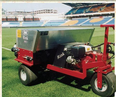
The redesigned self-propelled Rink 1015 has a large working width of 59" (1.5 m), what enables it to cover an area in a minimal amount of time. It's stainless aluminum steel hopper has a capacity of 18 cu ft (0.5 cu m) when filled level at the top of the hopper. The strong 13 hp Honda engine enables it to cover large areas quickly, while the 1015's 4 large tires are pivoting, so that ground contours are followed smoothly.
