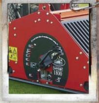
The Verti-Knife 1800 is a multi-functional tool that uses four sets of cutting discs on a rotating cartridge at variable spacing and depths. It is the ultimate root zone management tool for all surfaces and can work at depths from 0-6" at high working speeds.
