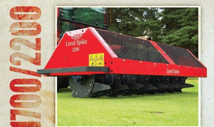
The Level-Spike is built tough and can be operated at speeds of 8.7mph (14 kmh) or more. The choice of available widths enables the customer to match the machine to their tractor and their specific requirements. There is an exceptionally wide range of knife options. There is an optional hydraulic weight transfer system which utilizes the tractor's hydraulics to force the tines into the ground providing maximum aeration and drainage.
